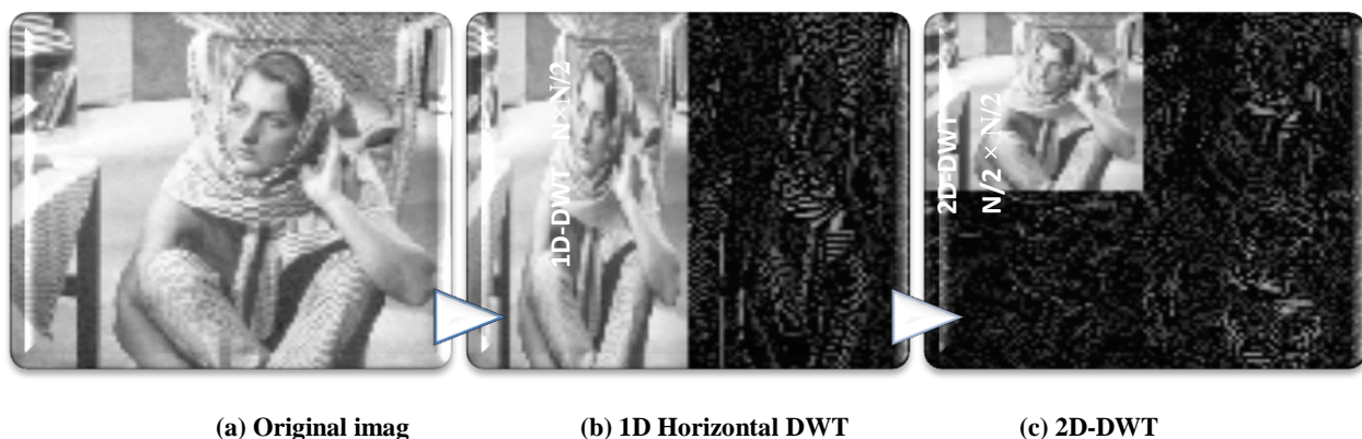
Fig. 7: the four subbands of forward 2-D DWT.
